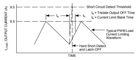
Figure 7. PWM Current Limiting Detail
