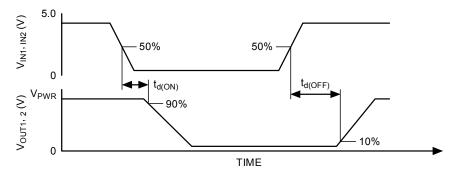
Figure 2. Output Delay Time
