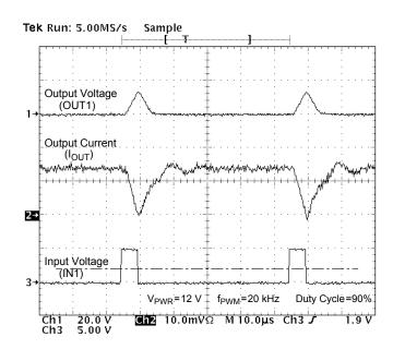
Figure 15. Output Voltage and Output Current vs. Input Voltage at V<sub>PWR</sub>=12 V, PMW Frequency of 20 kHz, and Duty Cycle of 90% for a Purely Resistive Load
