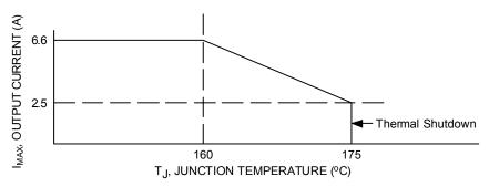
Figure 5. Output Current Limiting Versus Temperature (Typical)
