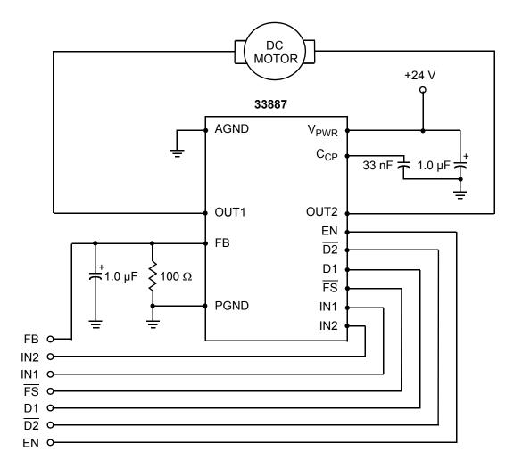
Figure 16. Typical Application Schematic
