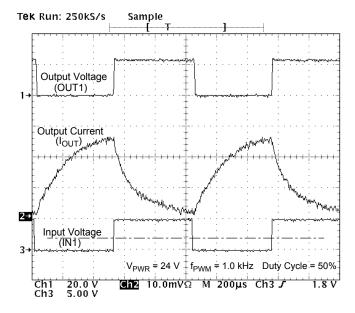
Figure 9. Output Voltage and Output Current vs. Input Voltage at V<sub>PWR</sub>=24 V, PMW Frequency of 1.0 kHz, and Duty Cycle of 50%
