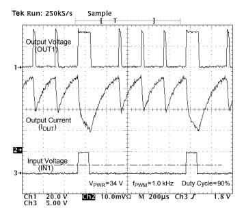
Figure 10. Output Voltage and Output Current vs. Input Voltage at V<sub>PWR</sub>=34 V, PMW Frequency of 1.0 kHz, and Duty Cycle of 90%, Showing Device in Current Limiting Mode
