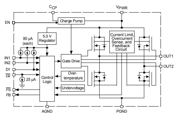
Figure 1. 33887 Internal Block Diagram
